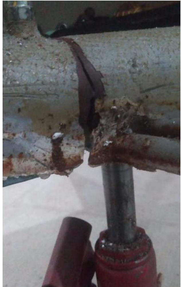
Figura 1 – Trincas no tubo de aço 4130 localizado no trem de pouso principal Figure 1 – Cracks in the steel tube 4130 situated in the main landing gear
