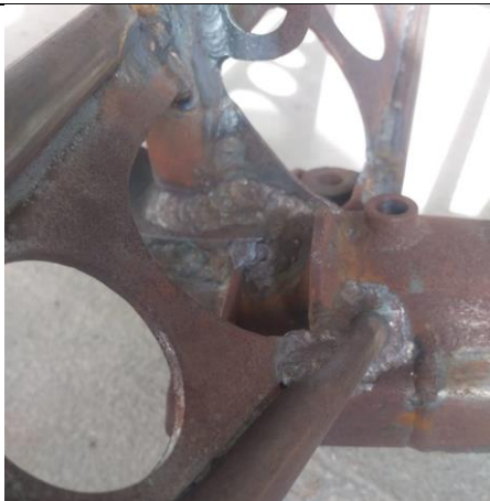
Figura 1 – Trincas no tubo de aço 4130 localizado no trem de pouso principal Figure 1 – Cracks in the steel tube 4130 situated in the main landing gear
