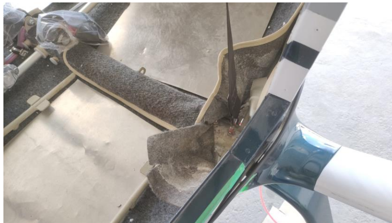
Figura 7 – Retirar o carpete que reveste o tubo central Figure 7 - Remove the carpet covering the central tube
